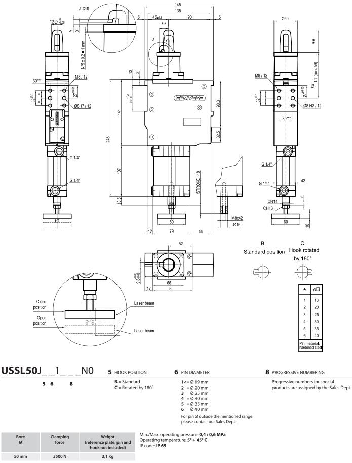
\*\* : MISSING DIMENSION TO BE DEFINED ACCORDING TO CUSTOMER SPECIFICATIONS \*\*\* : TOLERANCE BETWEEN DOWEL HOLES  $\pm$  0,02, BETWEEN SCREW HOLES  $\pm$  0,1
