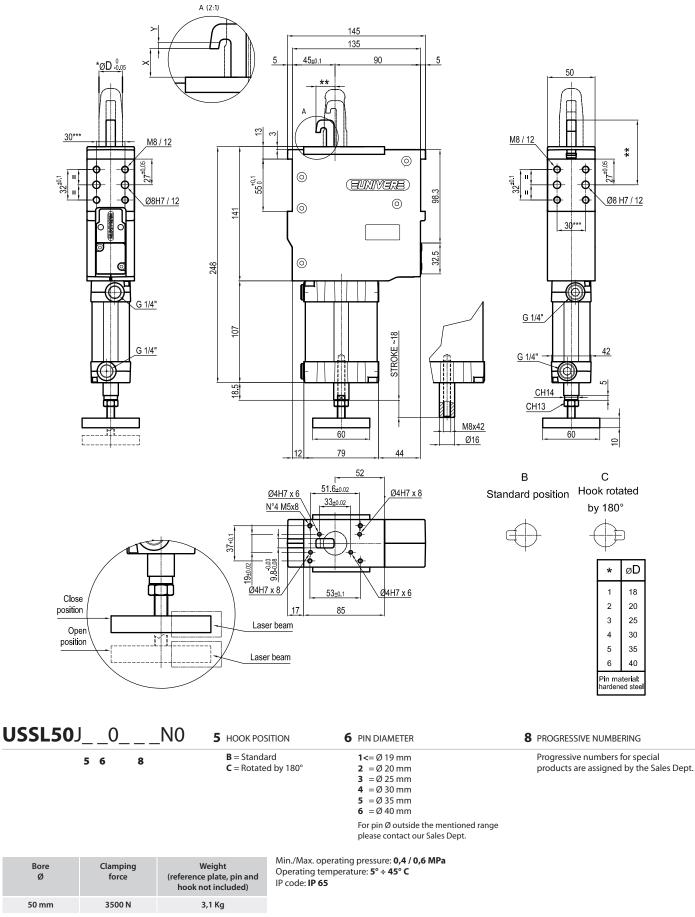
\*\* : MISSING DIMENSION TO BE DEFINED ACCORDING TO CUSTOMER SPECIFICATIONS \*\*\* : TOLERANCE BETWEEN DOWEL HOLES  $\pm$  0,02, BETWEEN SCREW HOLES  $\pm$  0,1 X= metal sheet
