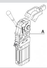
Mount self-holding group (C) on the fi xing block (A) without completely loose the nut (1).
