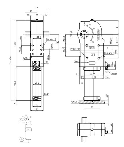
\*TOLERANCE BETWEEN DOWELS ± 0,02 BETWEEN SCREW HOLES ± 0,1 \*\*AREA TO ACCESS ANGLE ADJUSTMENT \*\*\*SCREW THREAD INSERT
