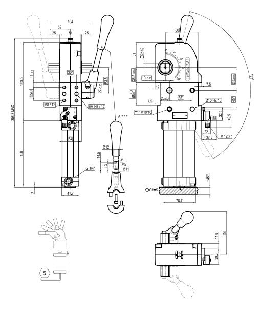
\*TOLERANCE BETWEEN DOWELS ± 0,02 BETWEEN SCREW HOLES ± 0,1 \*\*AREA TO ACCESS ANGLE ADJUSTMENT \*\*\*DIMENSIONS TO BE RESPECTED IN CASE OTHER MANUAL LEVERS ARE USED \*\*\*\*SCREW THREAD INSERT
