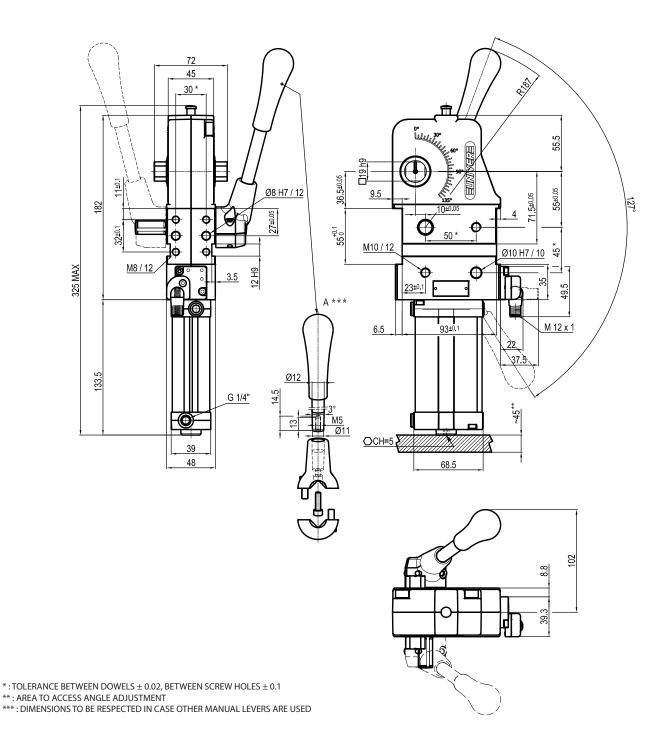
Cylinder bore Holding Clamping moment Weight Ø (0,5 MPa) (clamping arm not included) 50 mm 40 mm 1250 Nm 170 Nm
