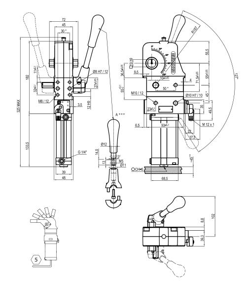
\*TOLERANCE BETWEEN DOWELS ± 0,02 BETWEEN SCREW HOLES ± 0,1 \*\*AREA TO ACCESS ANGLE ADJUSTMENT \*\*\*DIMENSIONS TO BE RESPECTED IN CASE OTHER MANUAL LEVERS ARE USED
