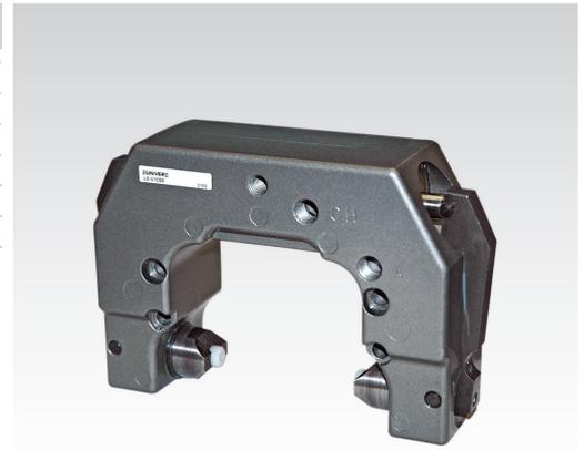
UNIVER Locking Units for rodless cylinders perform the function of keeping the carriage in any intended point of its stroke and allow high locking accuracy. They can be mounted on both sides of the carriage and the mechanical braking force can be further increased by means of an additional pneumatic override.
