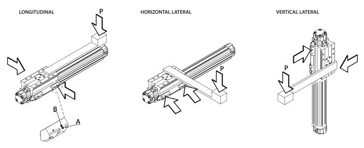
The arrows indicate the screws to be adjusted, based on the position of the load (P). Turn the screw (A) according to the load. Put a drop of Loctite 242 onto the screw (B) and tighten it all the way down. Finally loosen both screws by 90°.
