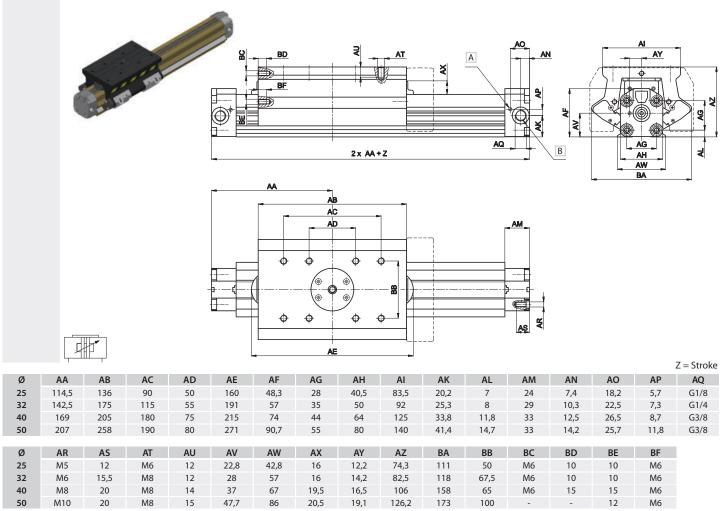
The dimensions of the L6 locking unit are indicated by dotted lines; for the fixing holes of the locking unit, see dedicated chapter.
