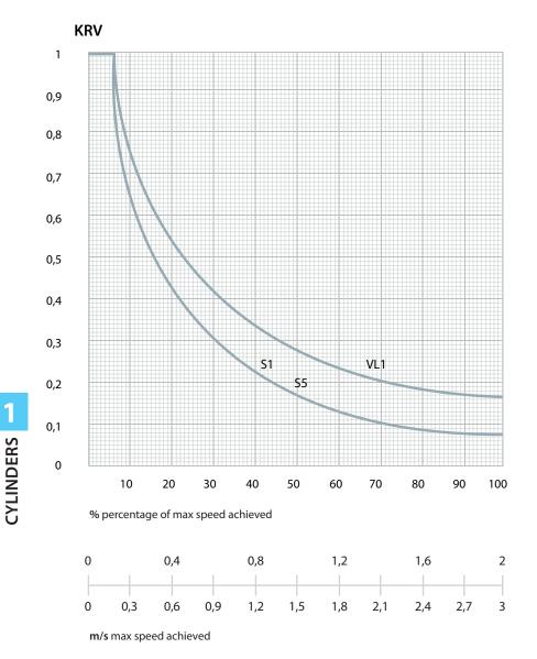
1) Calculation of the operational speed percentage in relation to the max allowable speed:
