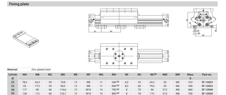
800 (a) 50 136 115 133,7 15 M10 14 70 60 8 115 (a) = Max allowable dimension to limit the bending of the cylinder according to the stroke and to provide a correct fixing
