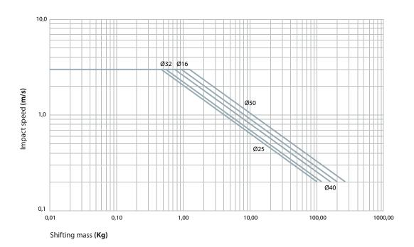
As a result, if cushionings can not absorb the kinetic energy and changing the working parameters is not possible, it is necessary to provide an additional hydraulic shock absorber (YDA / YDR series) to reduce the load speed before the cushionings operate.
