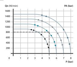
P = Working pressure PA = Supply pressure Qn = Flow rate
