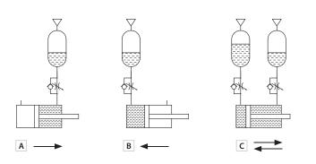
A-B-C = Regulation direction of piston rod's speed
