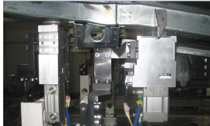
Pneumatic Power Clamps and Pin Clamp applications
