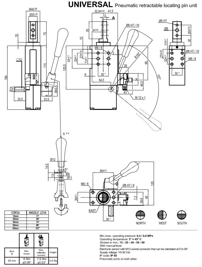
\* : TOLERANCE BETWEEN DOWEL HOLES ± 0.02, TO SCREW HOLES ± 0.1 \*\* : DIMENSIONS TO BE RESPECTED IN CASE OTHER MANUAL LEVERS ARE USED
