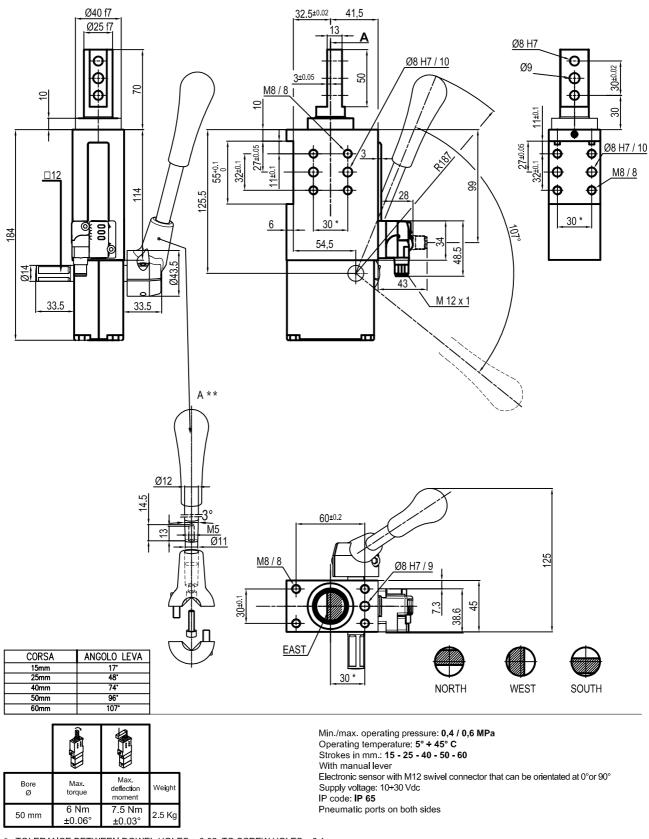
\* : TOLERANCE BETWEEN DOWEL HOLES ± 0.02, TO SCREW HOLES ± 0.1 \*\* : DIMENSIONS TO BE RESPECTED IN CASE OTHER MANUAL LEVERS ARE USED
