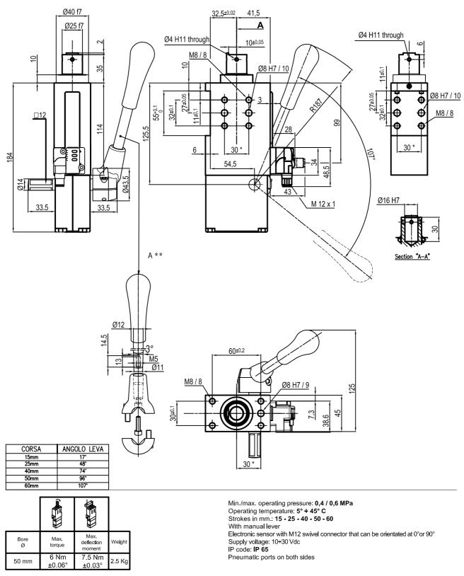
\* : TOLERANCE BETWEEN DOWEL HOLES ± 0.02, TO SCREW HOLES ± 0.1 \*\* : DIMENSIONS TO BE RESPECTED IN CASE OTHER MANUAL LEVERS ARE USED
