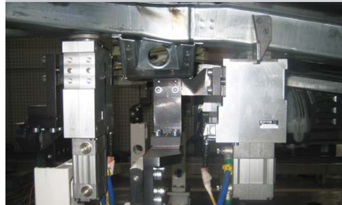
Pneumatic Power Clamps and Pin Clamp applications
