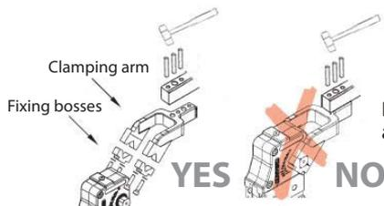
**Do not insert the dowels in the clamping arm when it is assembled on the clamp**
