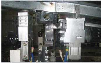
Pneumatic Power Clamps and Pin Clamp applications
