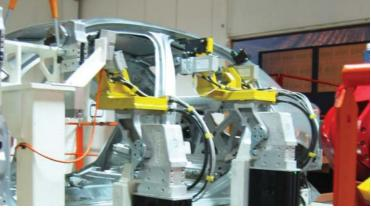
Pneumatic and electric Power Clamp applications
