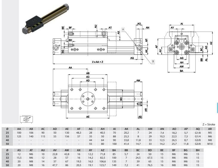
Dimensions of the L6 locking unit are indicated by dotted lines; for the fixing holes of the locking unit, see dedicated chapter.
